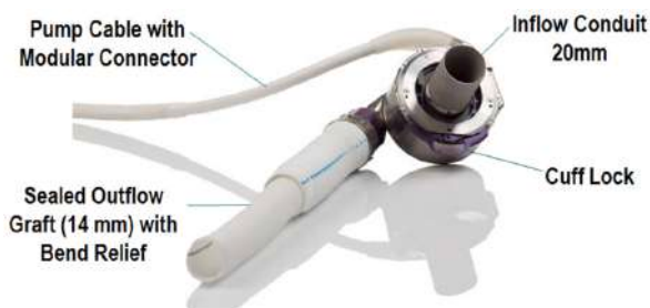
Figure 29: HeartMate 3 LVAD pump
